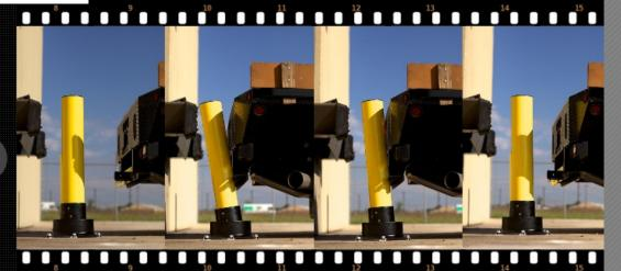
Rigid fixed protection bollards and concrete structures still often cause unnecessary damage to vehicles, the bollards themselves, or even to the objects that need protection. Thanks to the SlowStop® Bollard dynamic protection system, you can easily avoid this now. SlowStop® drastically reduces your costs because the risk of accidents causing vehicle, material, asset or facility damage is avoided while reducing the chance of personal injury.
